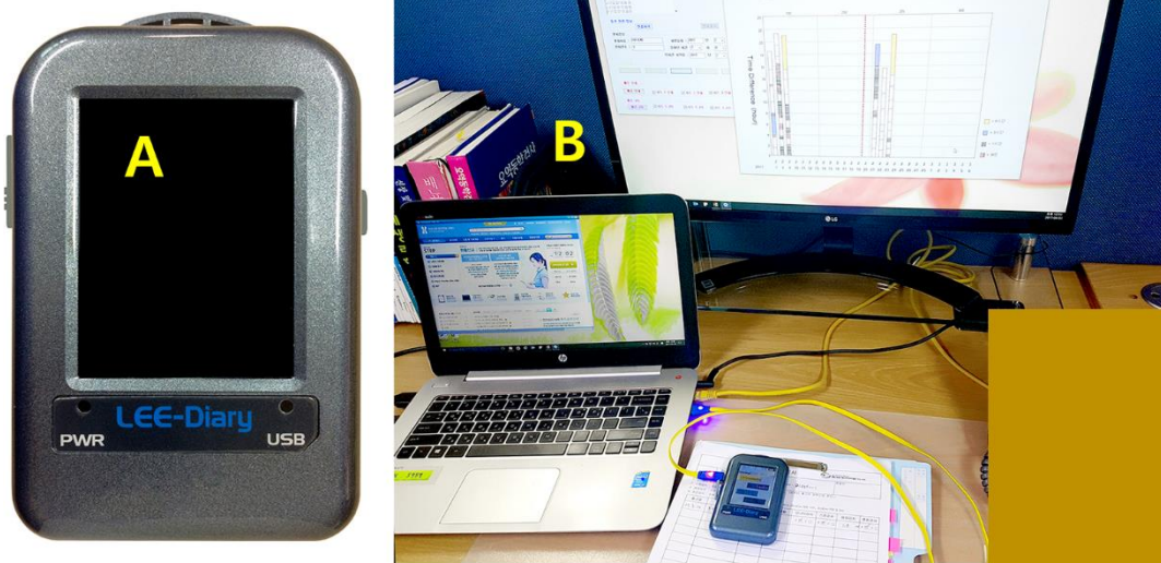
Fig. 1. Electronic Voiding Diary (VD). A. Image of electronic VD, (size: 64(W) x 95(H) x 15.5(D) mm). This has 2.4 inch touch screen to record the data related to micturition. B. If electronic VD is connected to computer via USB cable, various style of analysed results are automatically displayed on the computer screen.
